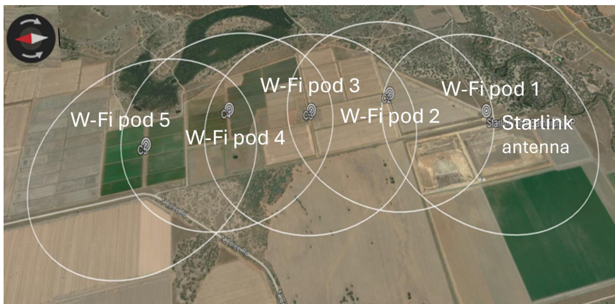
Figure 2 Illustration of the Wi-Fi MESH network at RRAPL consisting of a Starlink antenna to provide the site with internet and five Wi-Fi pods to spread the signal over ~958 ha.
