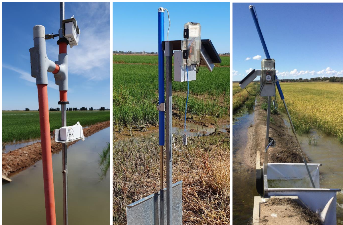
Figure 2 Illustration of a float (left), automated stainless steel slide door (middle) and automated tarp insert door (right) used in the case study.
