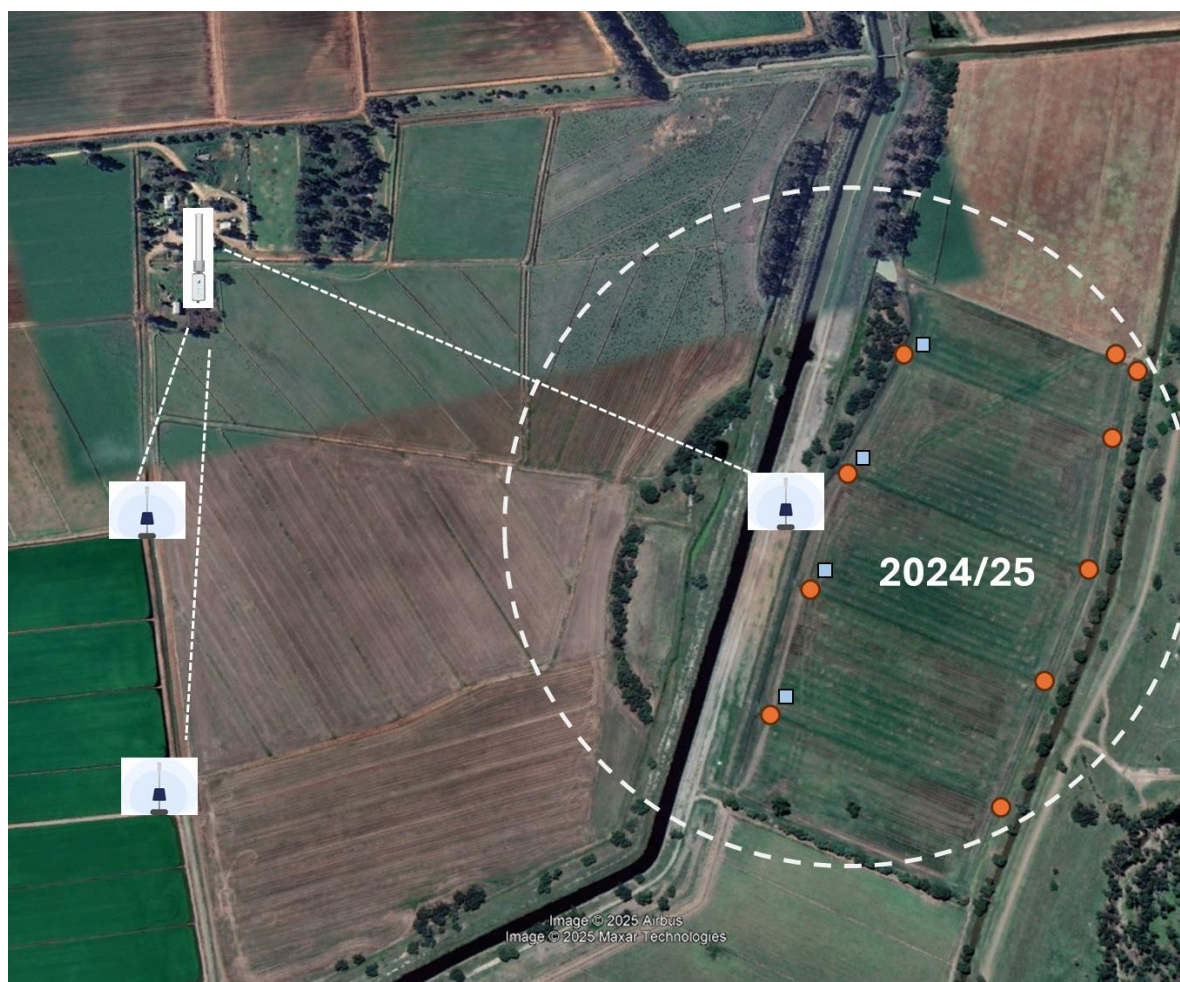
Figure 4 Illustration of the farm at Gogeldrie where bays were equipped with irrigation automation technology in the 2024/25 rice growing seasons. Location of the Wi-Fi Point to MultiPoint antenna (in the farmhouse) and Wi-Fi pod and its coverage is shown. The red dots indicate outlets equipped with the smart Wi-Fi controllers 'Alfies' (orange circles), and floats (blue squares) aside to manage irrigation water based on water level on bays.
