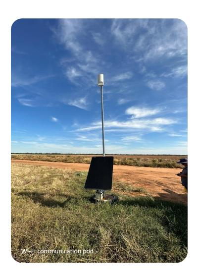
The communication pod is constructed using a sturdy metallic structure designed to accommodate the solar panel, battery, and Wi-Fi radio, elevated approximately 5 meters above the ground. The base of the pod utilizes a durable UTE or tractor tire. Within the pod box, situated behind the solar panel, you will find essential components such as the solar regulator and PoE injector, which efficiently power the Wi-Fi radio.
